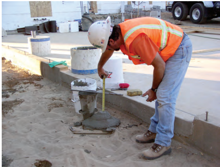
Figure 8.1 – Measuring concrete slump
