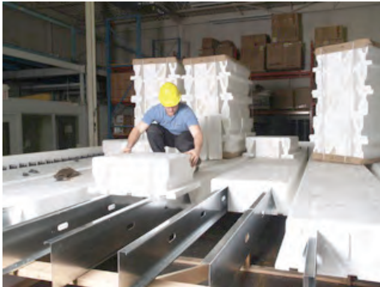
Figure 1.4 – Lightweight steel framing joists for the AmDeck™ floor and roof system
