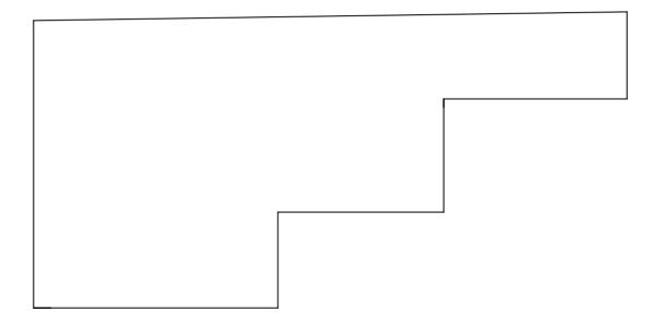
The largest portion of the structure that can be divided into a perfect rectangle is the western half. It would be most efficient to start in the southwest corner working north from left to right. The cut end at the end of the first row will be used to begin the next row.
